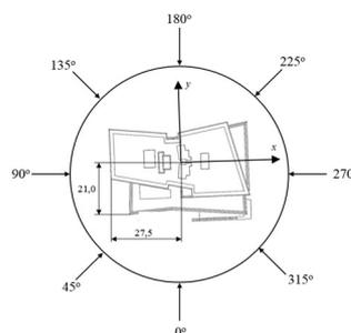
Fig. 1 – Building model and its surroundings: a) physical model in the working section of wind tunnel, b) location of the geometric centre and main wind inflow directions
